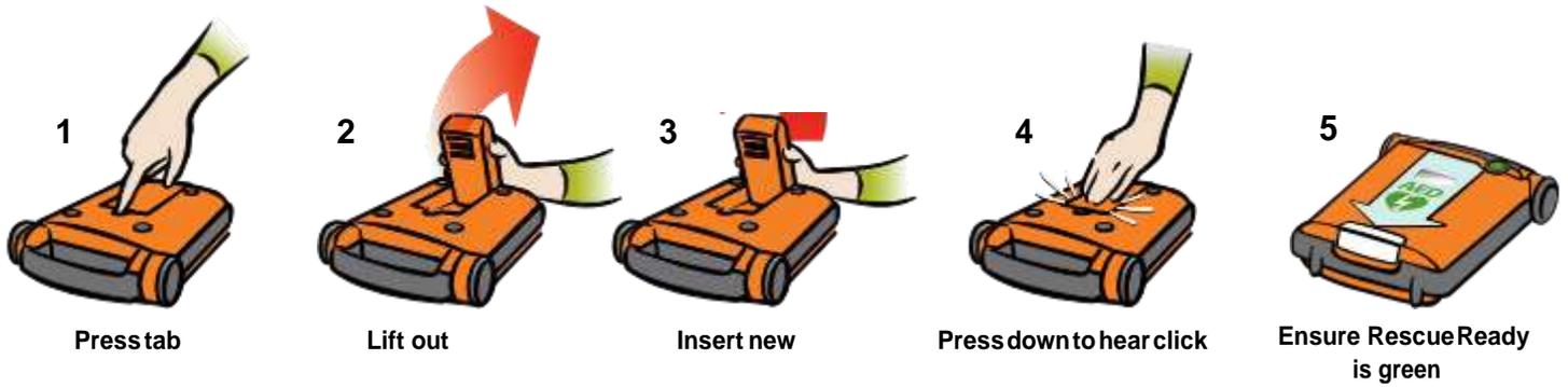
*Note: Ensure that the battery is at room temperature before inserting it into the AED.*
